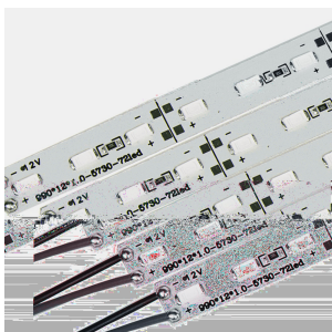
Figure 2 The LED modules which aren't requiring the additional cooling system [2]
